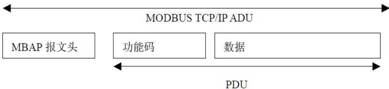
Figure 6: Request/Response of MODBUS on TCP/IP
