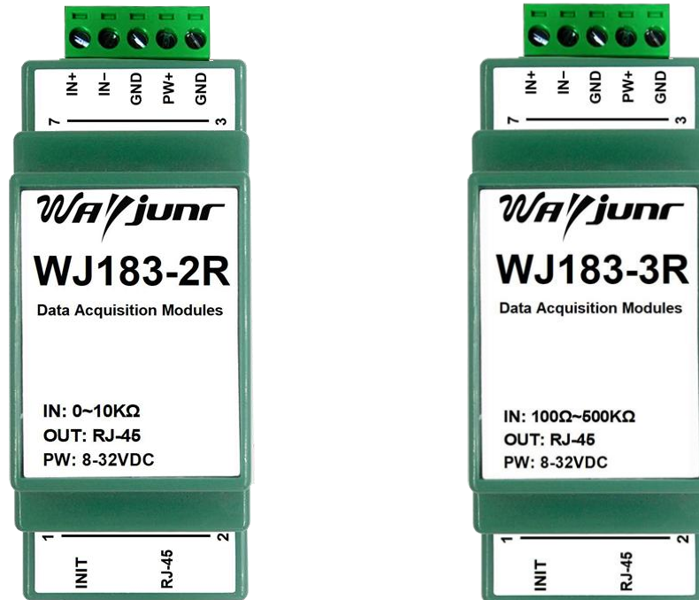
Two wire resistor, three wire resistor
