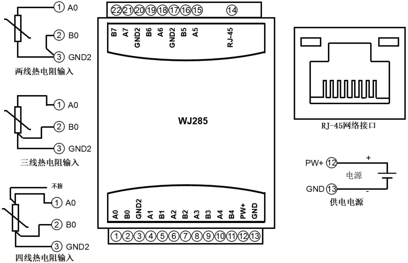
Figure 3 Wiring diagram of WJ285 module
