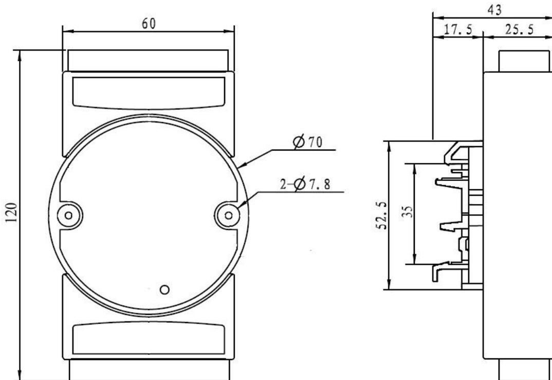
Can be installed on standard DIN35 rails
