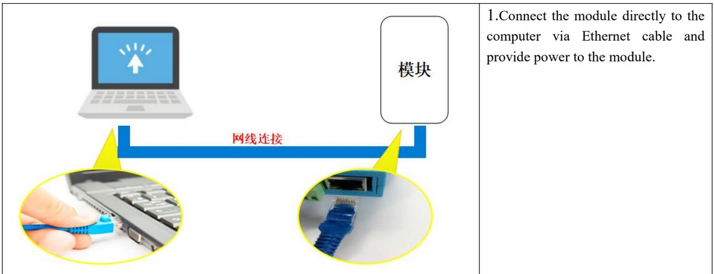
1. Connect the module directly to the computer via Ethernet cable and provide power to the module.
