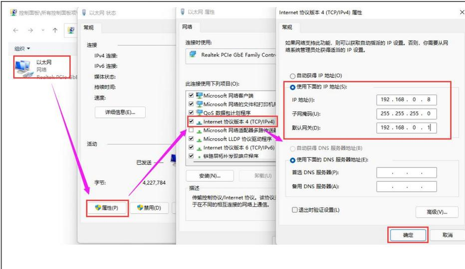
2. Open the computer "Ethernet" - "Properties" - "Internet Protocol Version 4 (TCP/IPv4)" - Set the computer IP and other information as follows:
