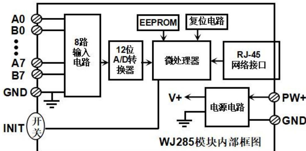
Figure 2 Internal Block Diagram of WJ285 Module
